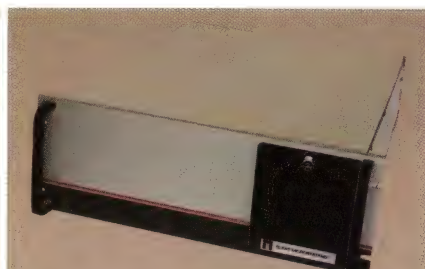
Rack mounted, rugged, 14 slot passive backplane, with 20 MHz 80386 CPU
